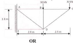
8 Determine the forces in all the members of the truss shown in Fig.
